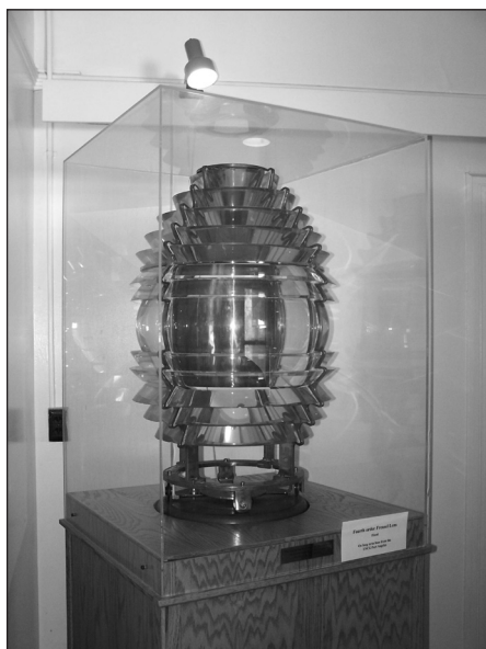
A fourth-order Fresnel lens, similar to that used at Monroe Harbor, on display at Admiralty Inlet Lighthouse, Washington. USLHS archive photo.
